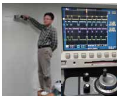
落下試驗 (2M高/各向/20次以上) Drop test (2M high/XYZ direction/20 times)
