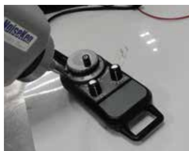
IEC耐靜電測試 (±10KV) IEC electrostatic discharge test (±10KV)
