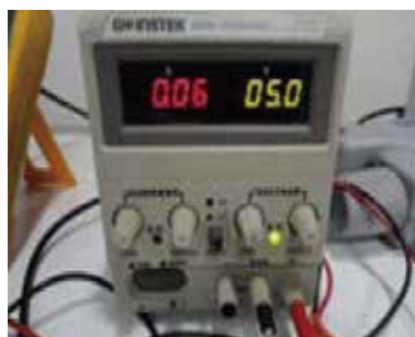
逆極性電壓測試 (36V/1min) Polarity voltage test (36V/1min)
